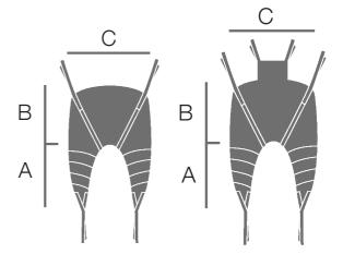
The widest part of the sling constitutes the back of this type of sling. The branches of the U constitute the thigh support.
